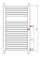
Lateral connections at connection centre personalized (2 manifolds + diaphragm)
