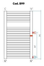
Lateral connections at connection centre personalized (2 manifolds + diaphragm)
