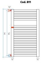
Couplings welded laterally in alignment with the first and the last element on the left side
